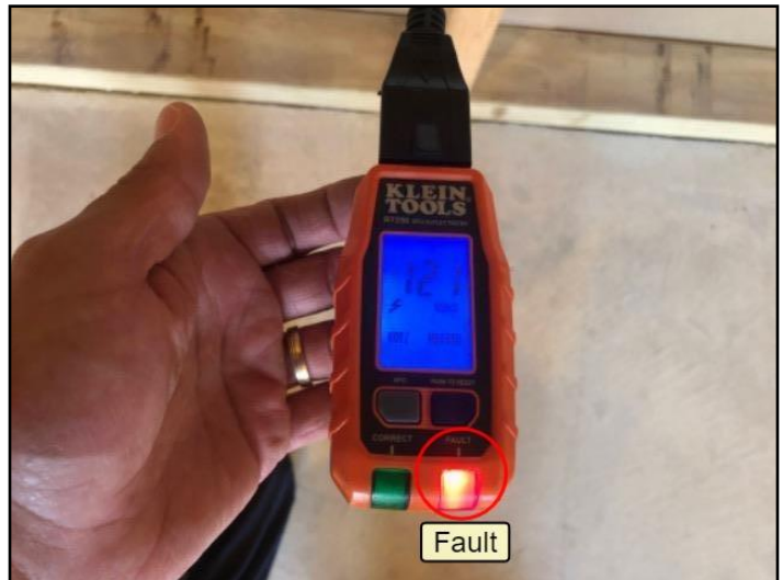
Improperly wired outlet, sample photo
