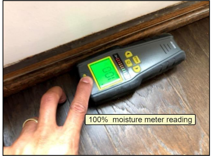
Tested wet (100%) checked with moisture meter
